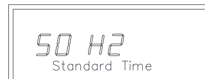
Frequency Setting Mode selected with frequency flashing. Use + and - to select required setting.
