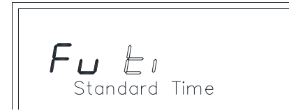
Function 'Time Setting Mode'. Press + three times to move to system settings
